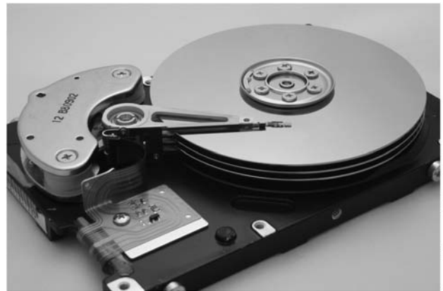
FIGURE 1.6 Computer hard disk drive, showing disks and read/write head
